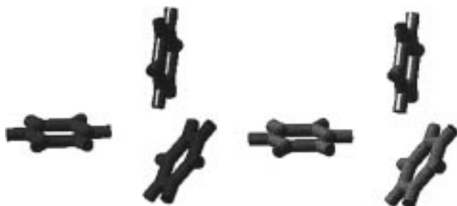
Figure 3. Benzene–benzene interactions in the microchannels of 1 ·1.5 benzene. The benzene molecules also interact with the walls of the microchannels.
